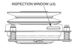
Figure 6-10. Clutch Air Gap Adjustment
